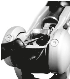
Fig 4. Remove head cap screw
